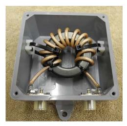
Install the supplied pipe clamps onto the Nema 4 enclosure, this is the common mode choke for the coax.
