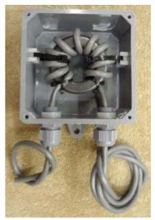
Remember: If the common mode choke is too small for the amount of RF power being generated, the ferrite material will saturate, become very hot and could break into two pieces! "We have seen 2.4 inch ferrites split under high reactive loads!" Once this happens common mode currents will flow on the control cable or coax outer shield. This can cause RFI problems, RF burns and could damage your antenna controller, regardless of make or model.
